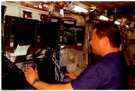
Figure 19 Portion of the workstation that allows controlling Canadarm2 on the ISS. The astronaut manipulates the robotic arm with two joysticks. He has to optimize the limited views offered by the three monitors. (Source: NASA)
