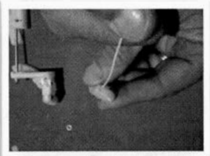
Figure 22: Thread the finger bungy 1
